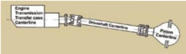
This illustration shows the proper geometry for a driveshaft featuring a double cardan joint and conventional U-joint.
