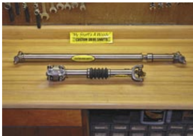
Front is a double cardan shaft with a conventional two-joint shaft in back. A reverse slip driveshaft (not shown) will have the slip yoke at one end. The reverse slip is the type of shaft used with the OE 231 transfer case.
