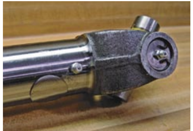
The slip joint in a driveshaft (left) is designed to accommodate changes in shaft "stroke" due to suspension and chassis flexing. As with the greasable U-joints (right), the slip joint must also be liberally greased to ensure proper operation.
