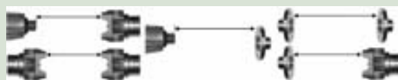
Here you can see the points for measuring driveshaft length, depending on your yoke configuration.
